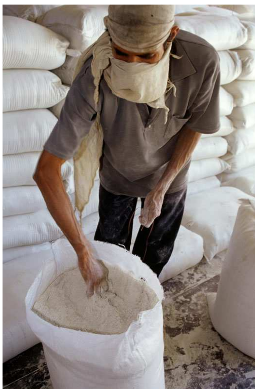
Figure 2 Worker in India handling asbestos with minimal respiratory protection. (Photo courtesy of P Madhavan).
